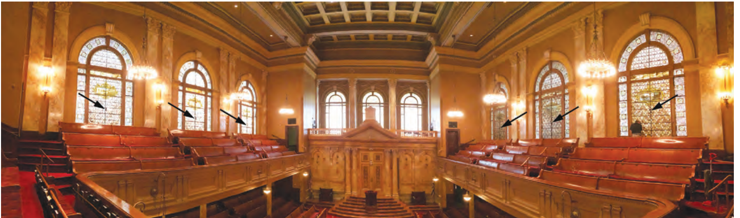
Fig. 8. Sanctuary with east windows removed and geophones in place (black arrows). Photograph by ANA, 2015.
