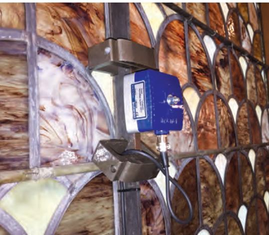
Fig. 6. Geophone mounted on a vertical stabilizing bar with custom clamps. Photograph by ANA, 2015.
