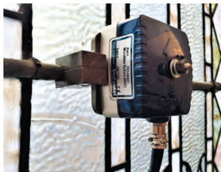
Fig. 7. Geophone mounted on a saddle bar with a custom clamp. Photograph by ANA, 2015.
